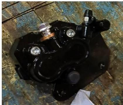
*Figura 15. Caliper de Italika ATV 250.*
