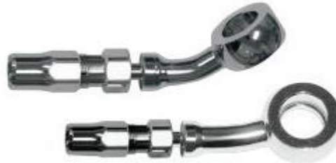
Figura 30. Banjo conector manguera – caliper [21].
